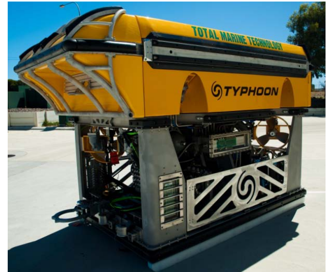
This ROV Utilises Matrix's Ultralight Carbon Fibre Syntactic Foam Buoyancy. *
